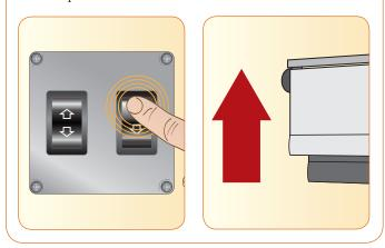
Fine-tune the Upper Stop Position by lightly pressing and releasing the Up switch until you reach your desired Upper Stop Position. Do not press the Down rocker switch only use the Up.
