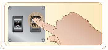
**F** Fine-tune your Lower Stop Position by lightly pressing and releasing the Down switch until you reach your desired Lower Stop Position. Do not press the Up rocker switch, only use the Down.
