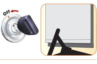
↓ With ignition power on, confirm that the shade stops at Ignition-On settings. With ignition power off, confirm that the shade stops at Ignition-Off settings.
