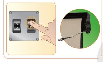
**C** While holding the wall switch in the Down position, press and hold the Programming Button until motor beeps. Hold until motor beeping stops. Release both.
